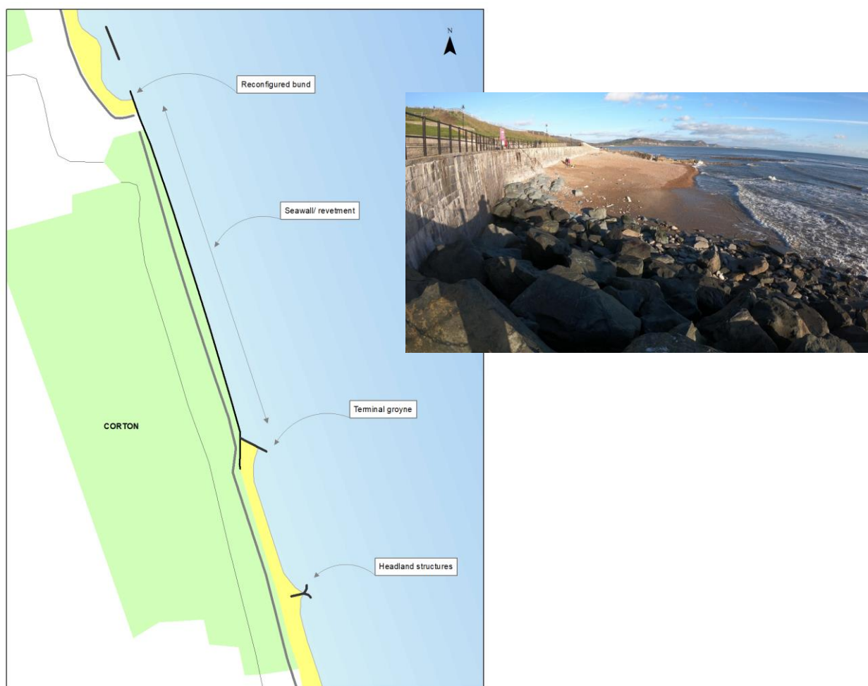
Figure 6-3: Illustration of how the proposed approach could look at Corton. The photograph shows an example of rock revetment in front of the main defence at Lyme Regis Church Cliff. Source: Love Lyme Regis Ltd 2021 ( https://lovelymeregis.co.uk/beaches/churchcliffbeach )
