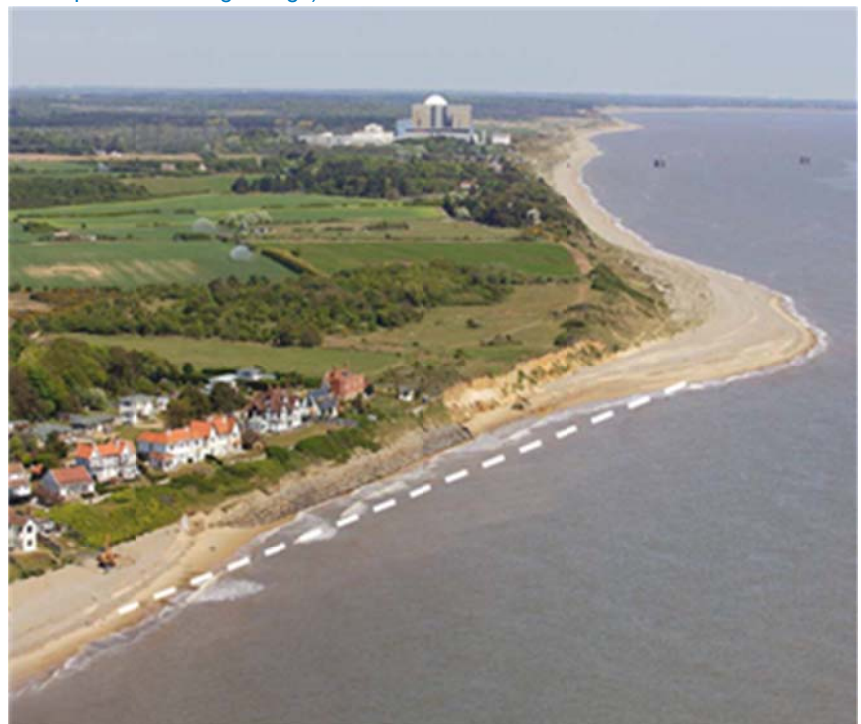
Figure 2.3: Beach set-back in front of coastal protection at Thorpeness (prior to the placement of geobags)
