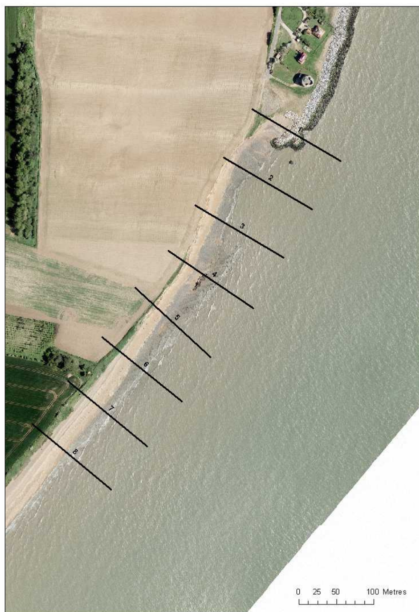
Figure 2.3. Location of coastal transects. Note the bay is present between profiles 1 and 4, but the London Clay shore platform extends between profiles 1 to 8.
