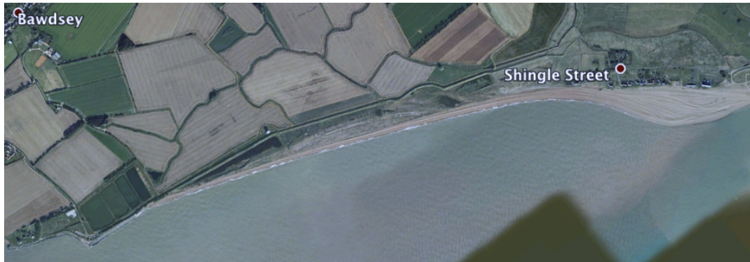
Fig.3: Google Image of SSB and SSN (2008) Note the swash-aligned barrier remnant behind the centre of SSB and the sub tidal shoal flanking SSN that is related to the flood orientated structures at the mouth of the Alde-Ore immediately to the RHS of the image.
