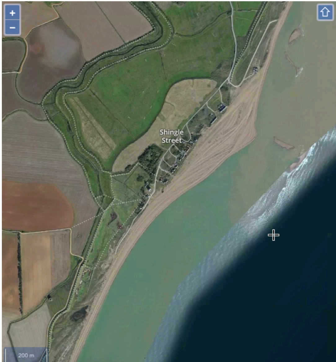
Fig.7E: SSN morphological structure as of 2017 (Google Earth) Note the early 21 st C. accretion to the northeast of the Ness that could be related to the increased dominance of northwards-directed transport identified by HR Wallingford (2016).
