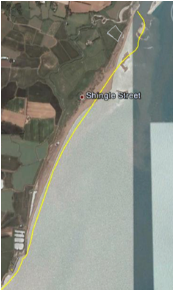
Fig.7D: SSB and SSN shoreline changes between 1945 (yellow) and 2013. Note the salient change in estuary mouth side bars plus growth of SSN.
