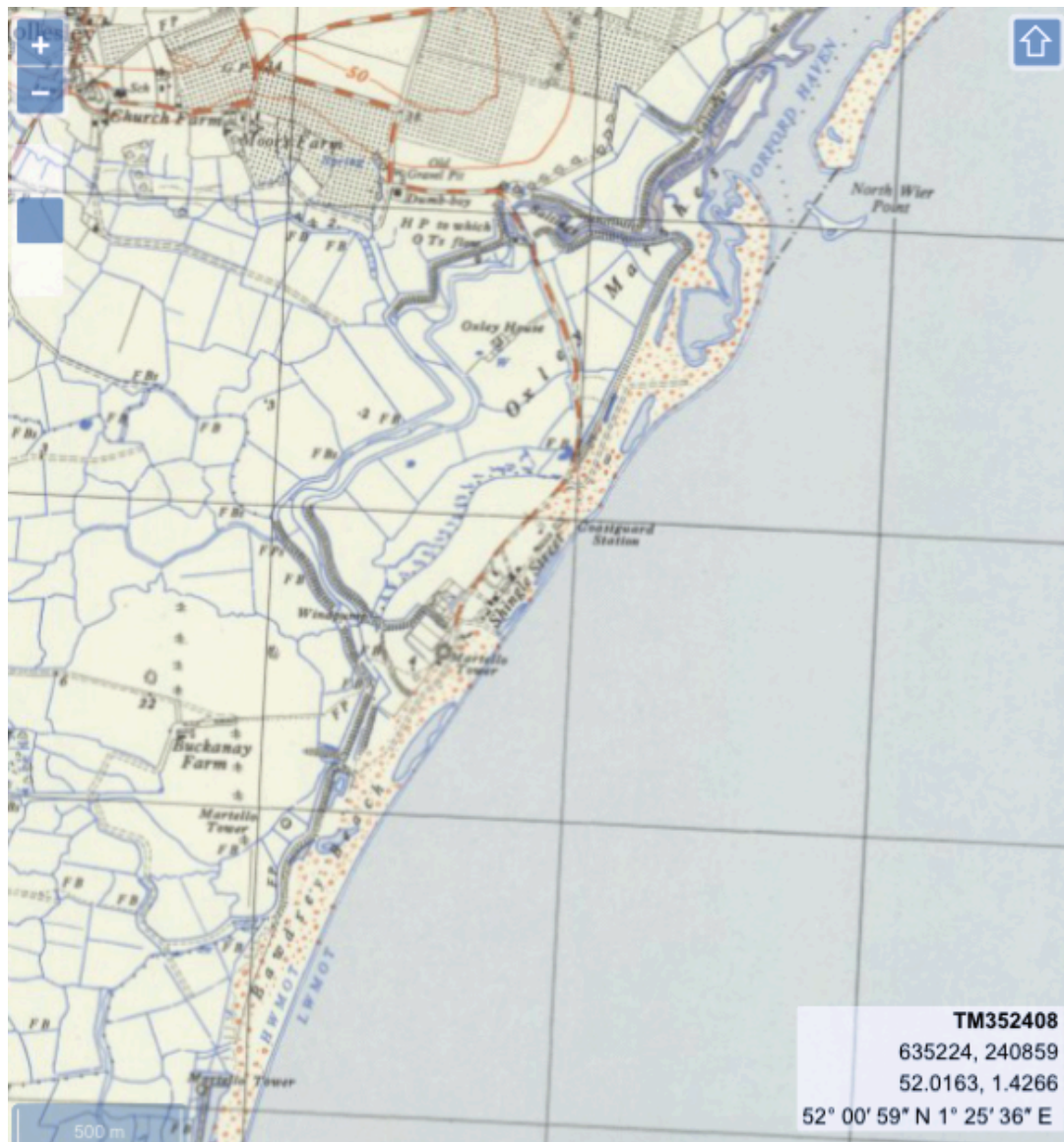
Fig.6: Section from OS 1:25000 available 1961. Note the lack of a ness at Shingle Street and the accompanying northerly directed spit at the Alde-Ore entrance as a reversal of structures at the mouth of the Alde-Ore exit (North Wier Point) compared to the early 20 th C. (cf. Fig.5).
