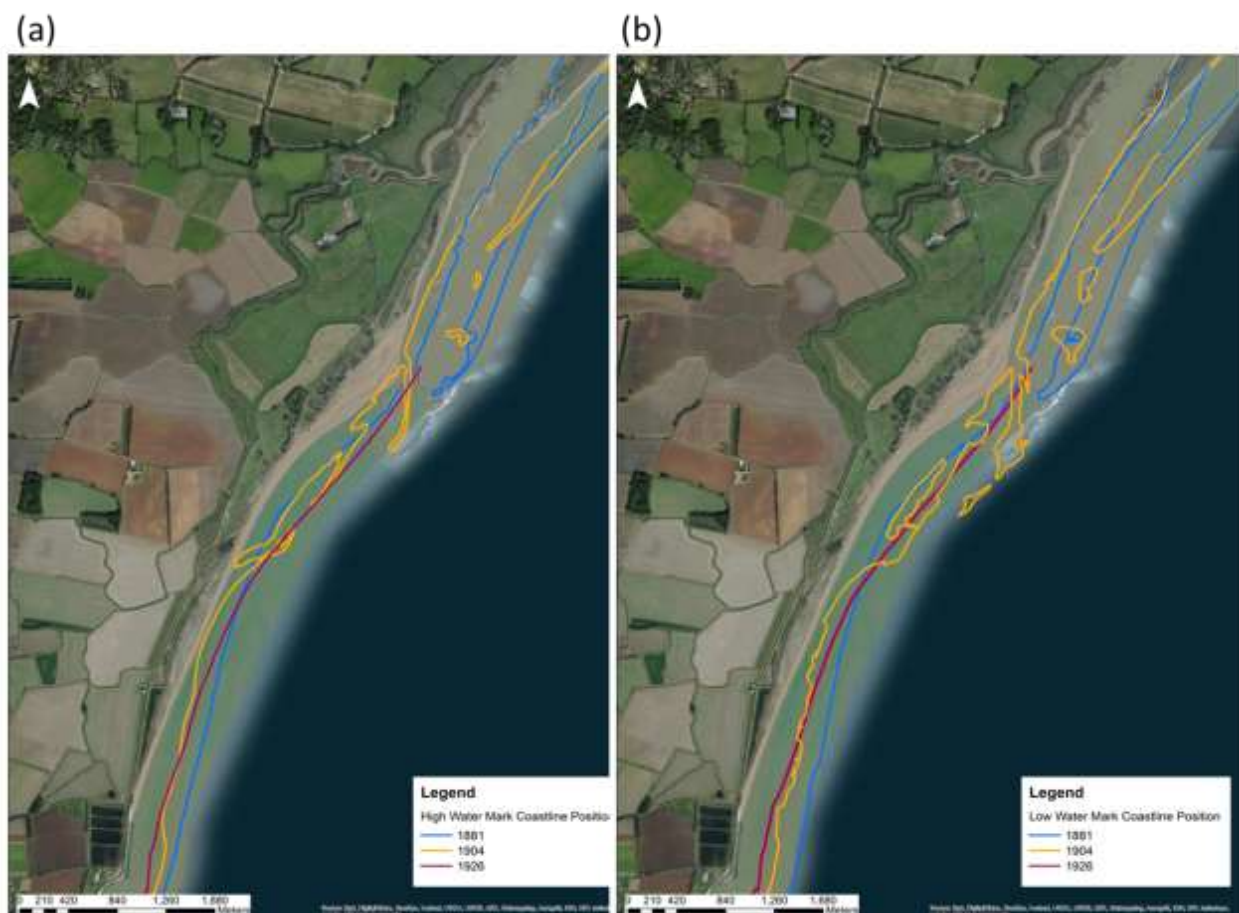
Figure 4.8: Historical changes in the Weir Point area between 1881 and 1926: (a) High water line; and (b) low water line.
