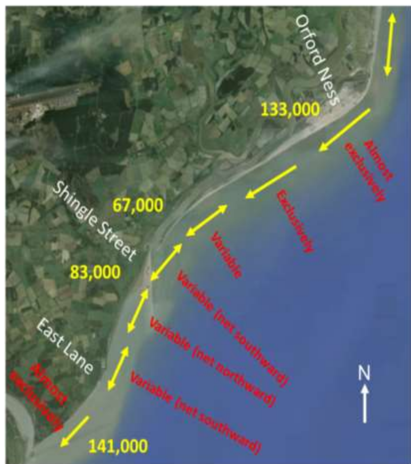
Figure 6.1 Schematic illustration of alongshore transport rates and directions
