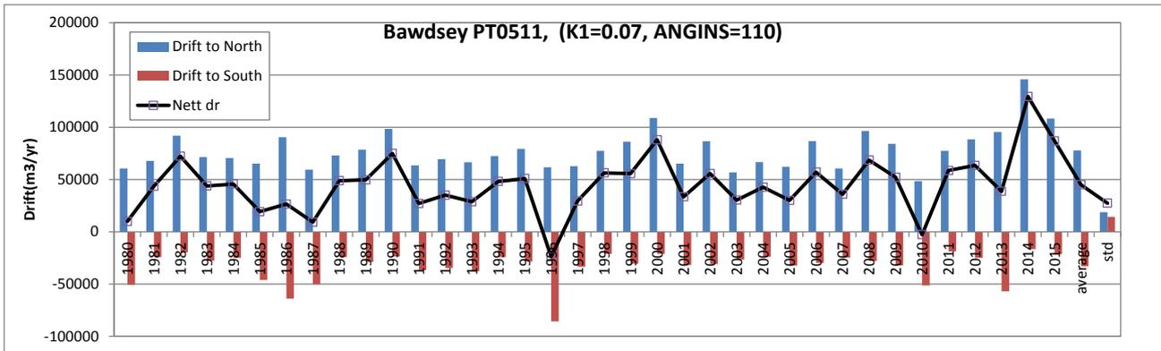
Figure G.2: Potential longshore drift from 1980 to 2015. Point PT0511
