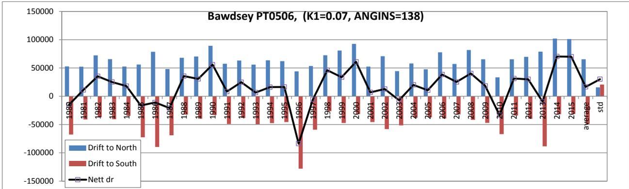
Figure G.7: Potential longshore drift from 1980 to 2015. Point PT0506
