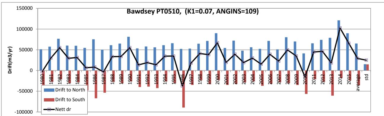
Figure G.3: Potential longshore drift from 1980 to 2015. Point PT0510
