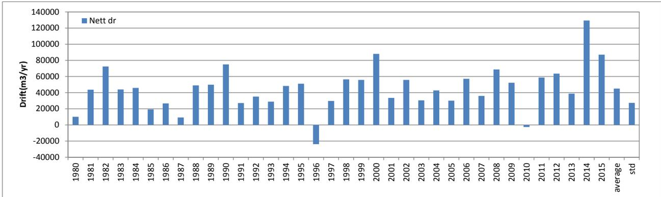
Figure G.10: Potential net longshore drift from 1980 to 2015. Point PT0511
