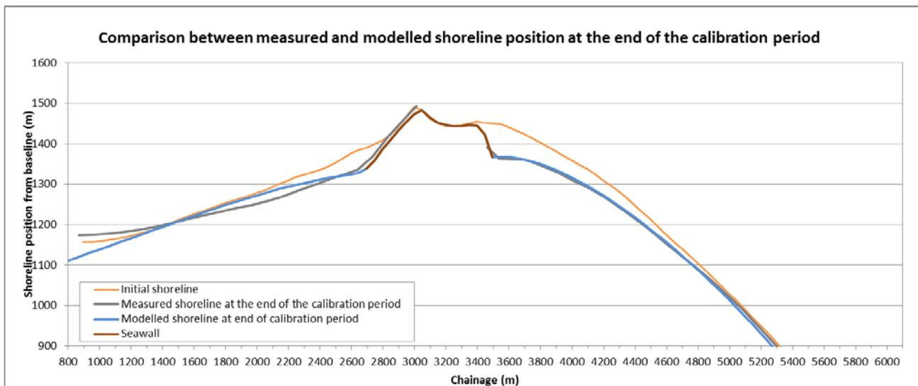
Figure 5.10: Comparison between measured and modelled shoreline positions at the end of the calibration period
