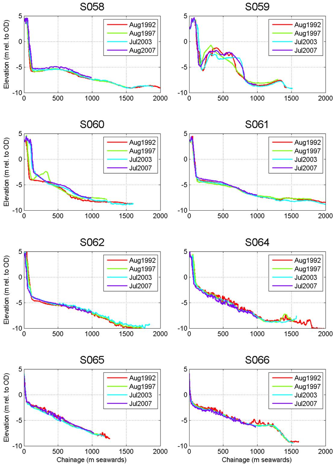
Figure 3.4: Comparison of long cross-sectional profiles (Ore/ Alde to Deben)
