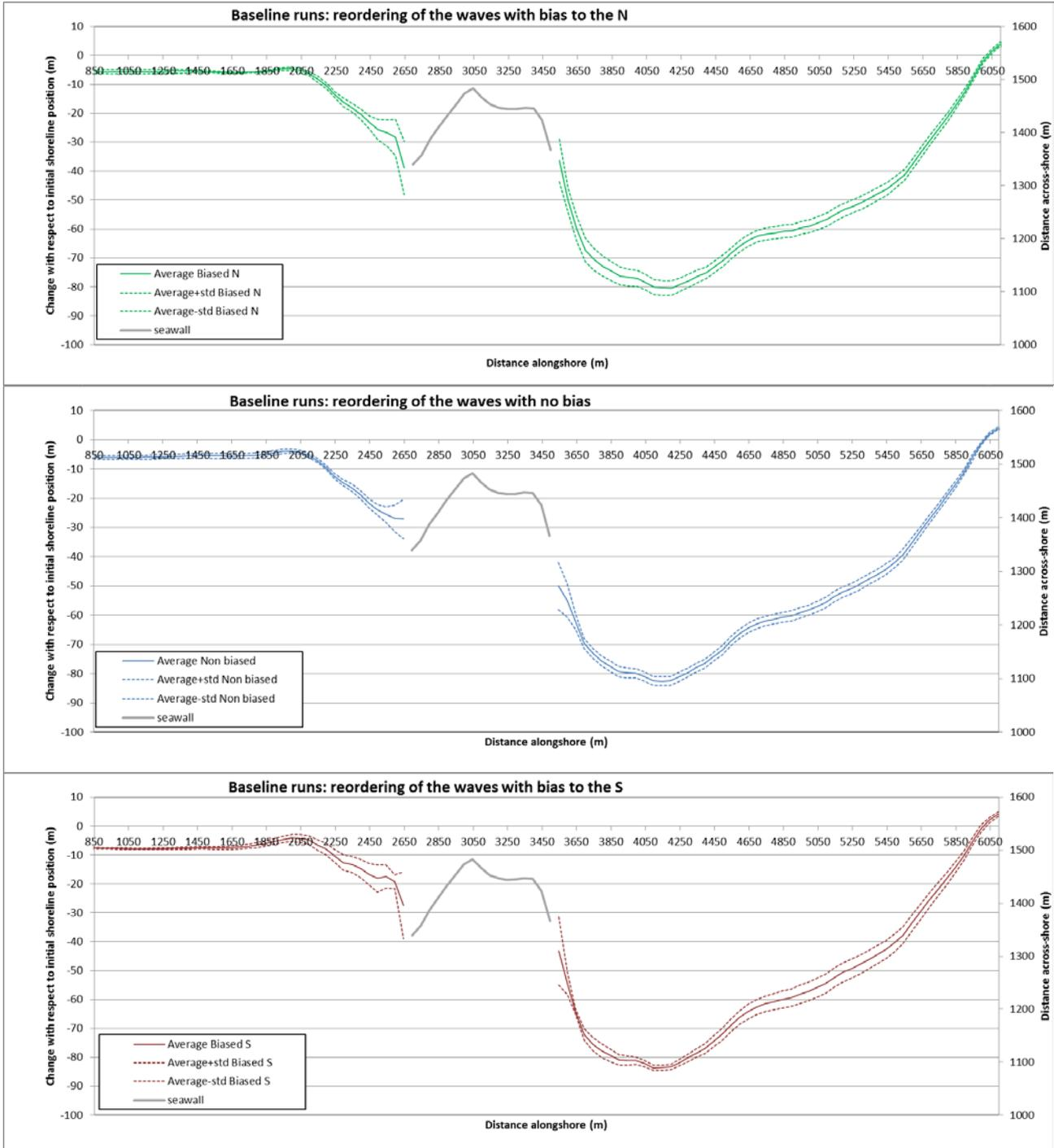
Figure H.4: Baseline runs: sensitivity to reordering of the waves, with or without bias
