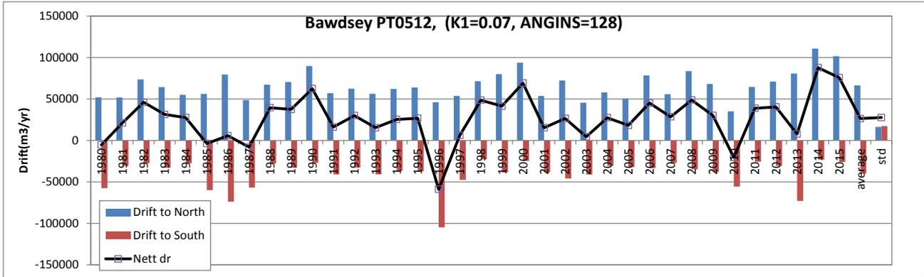
Figure G.1: Potential longshore drift from 1980 to 2015. Point PT0512 (S of Shingle Street)
