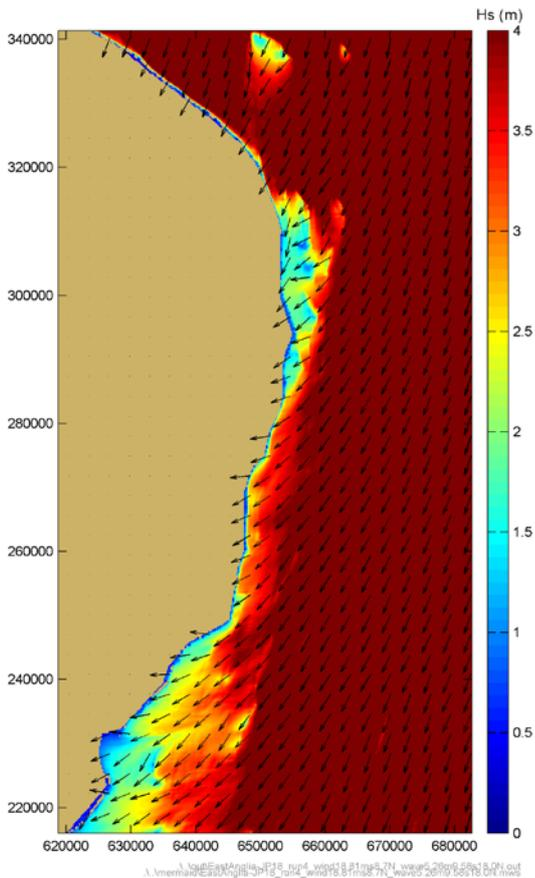
Figure C.3: Sample SWAN model output – predicted significant wave height and mean wave direction
