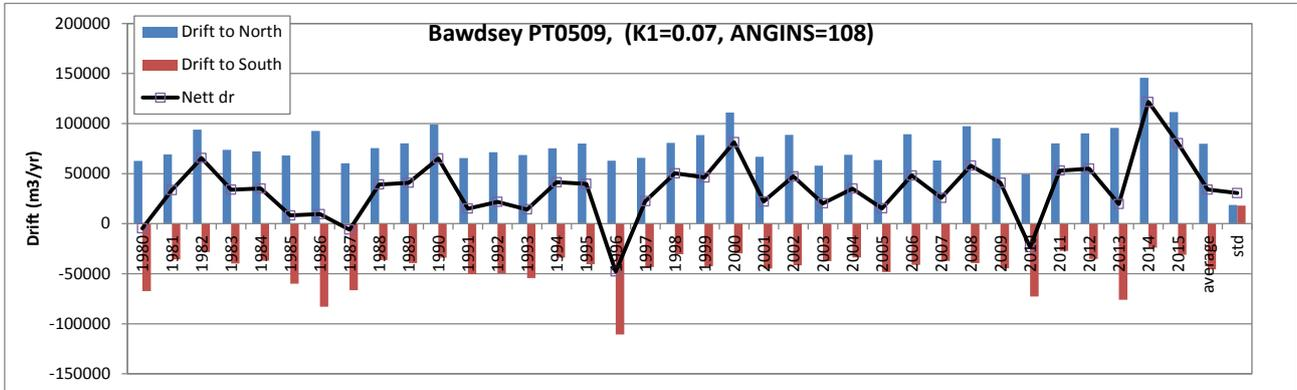
Figure G.4: Potential longshore drift from 1980 to 2015. Point PT0509 (East Lane)
