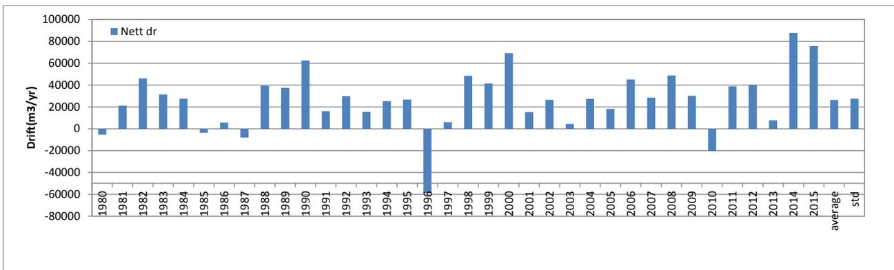
Figure G.9: Potential net longshore drift from 1980 to 2015. Point PT0512 (S of Shingle Street)
