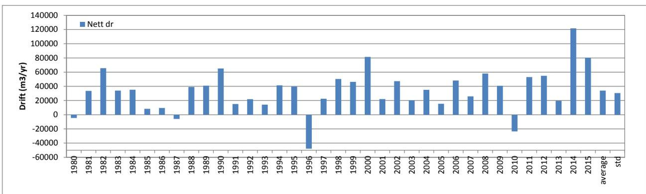
Figure G.12: Potential net longshore drift from 1980 to 2015. Point PT0509 (East Lane)
