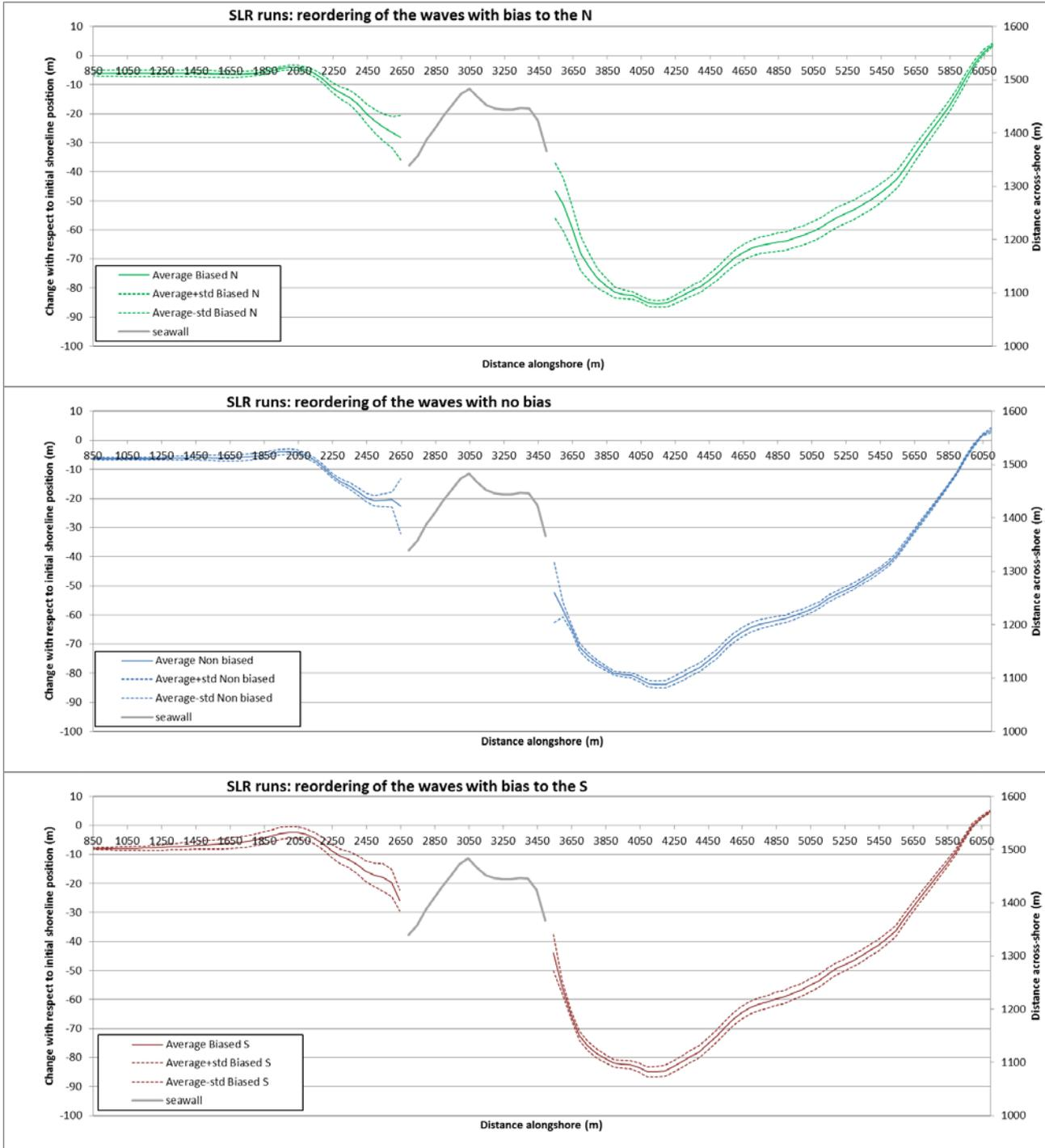
Figure H.8: S.L.R. runs: sensitivity to reordering of the waves, with or without bias
