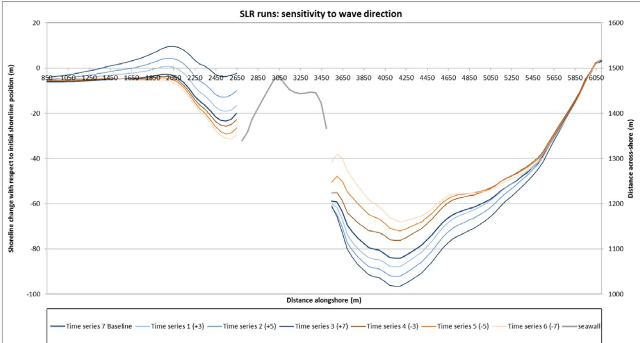
Figure H.7: S.L.R. wave conditions results: influence of rotating the wave direction
