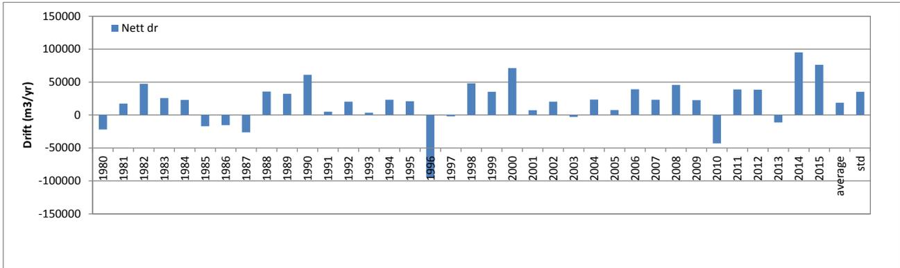
Figure G.13: Potential net longshore drift from 1980 to 2015. Point PT0508
