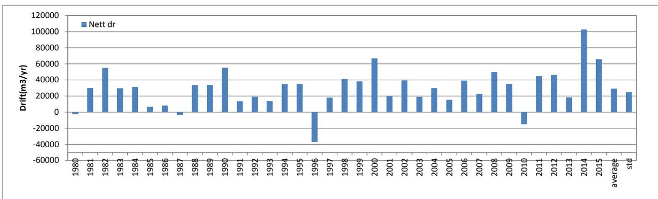
Figure G.11: Potential net longshore drift from 1980 to 2015. Point PT0510
