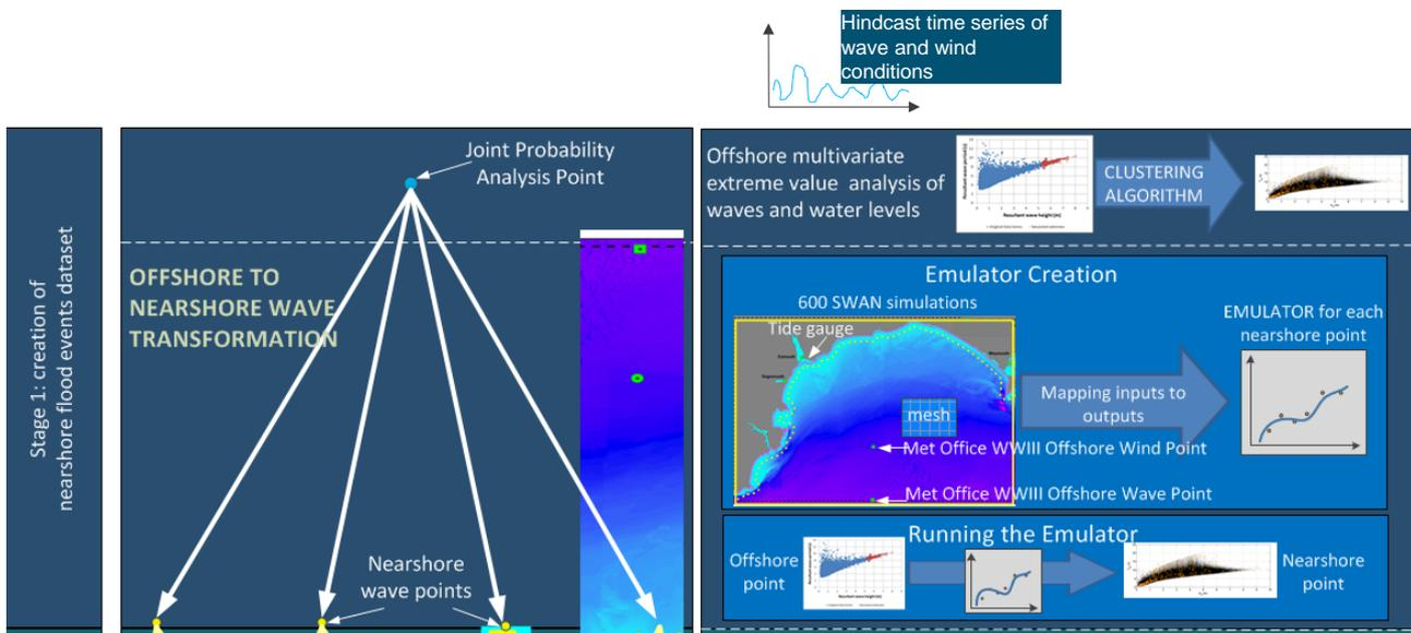
Figure C.1: Conceptual diagram showing the components of the analysis methodology
