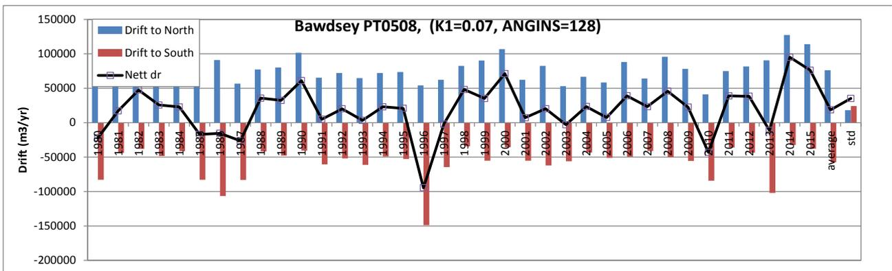
Figure G.5: Potential longshore drift from 1980 to 2015. Point PT0508
